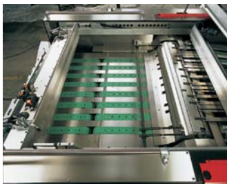
Synchronized belt speed to SPS® dryer: sheet transition without flutter and friction.
