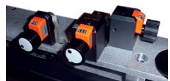
3-point screen fine adjustment units are centrally located on the operator side, equipped with central pneumatic locking and unlocking of the set position. The screen holder perfectly matches with pre-registration systems.
