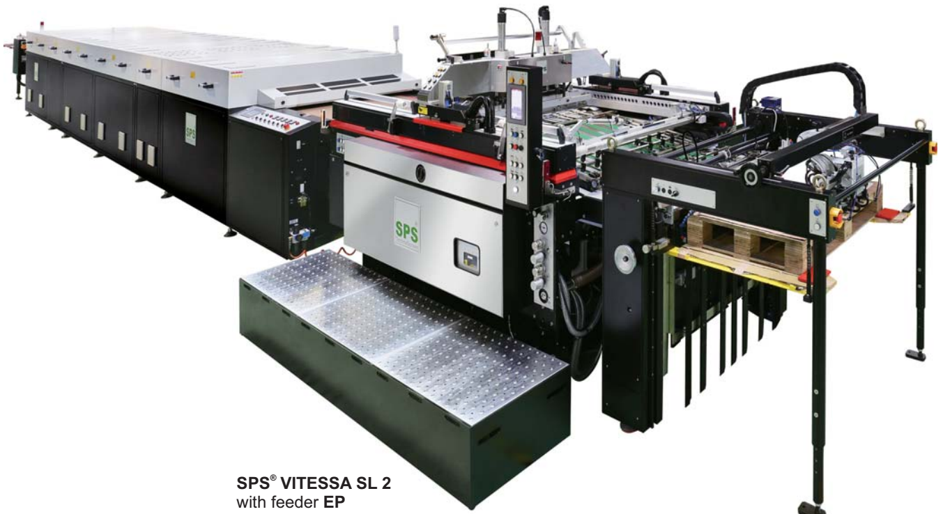
For screen change , the top frame is driven between the lifting posts into its raised position, and the inner carrier opens for the operator to pull out and push in the screen frames from the side.
