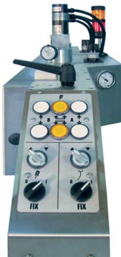
Motorized squeegee set-down. Squeegee blade change with automatic height leveling.
