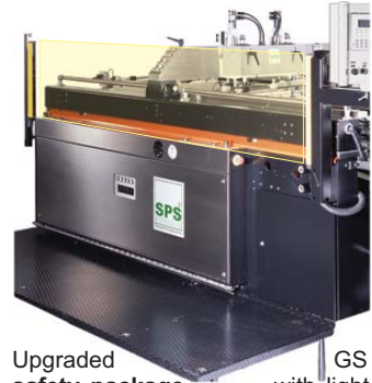
Vacuum side guide convertible: additional push function to align heavy substrates.
